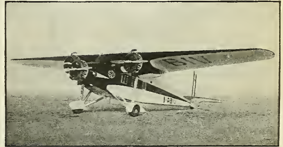
New Savoia-Marchetti —Italian ship, equipped with 35 x 15-6 Airwheel Tires and Hydraulic Brakes
